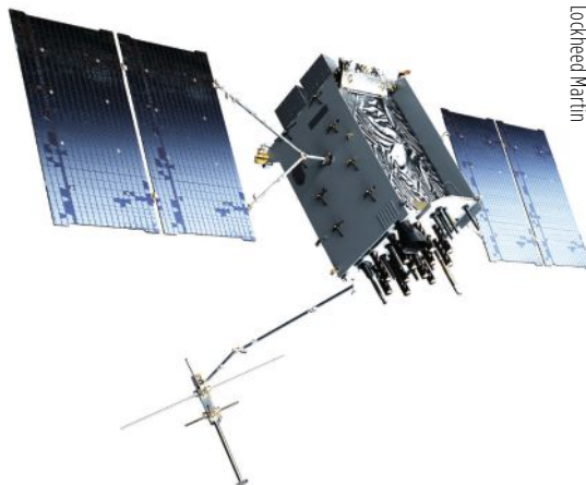
The GPS III satellite has additional anti-interference features.
