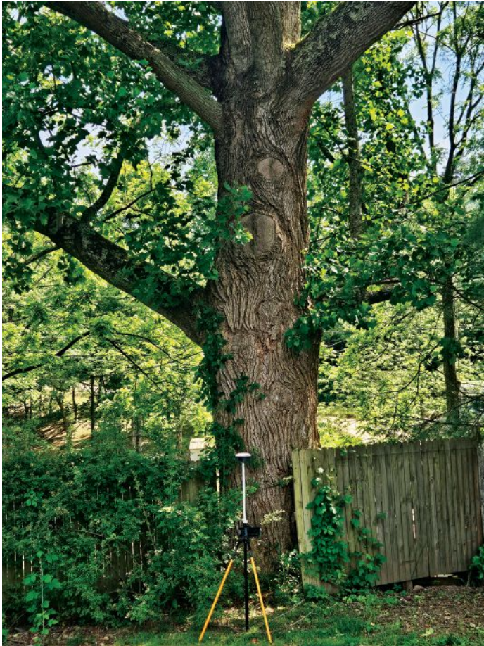
TREES , such as this 150 year old tulip poplar, were killers of previous generation GNSS systems. Robust designs, the modern sensor stack, and powerful algorithms can now fix reliably in heavy canopy, saving hours of traditional work.
